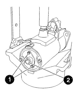
Disassembling commutator end shield
